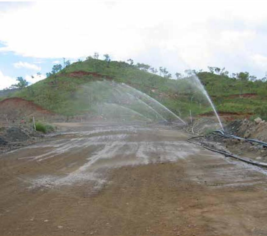
The Haul Road Spray System provides automated, high frequency, light watering of the haul road to prevent dust lift off. It does it without the high labour or equipment costs associated with water tankers.
